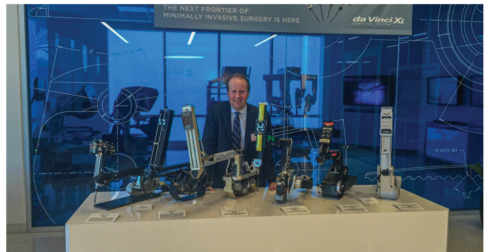
Figure 2. At Intuitive Surgical headquarters, they display their chronology of robotic platform arms from the various systems. Over the course of robotic platform and instrument upgrades, surgeons have access to longer instruments, articulating tips, and a library of different possibilities for cutting, grasping, sealing, and dissecting.
